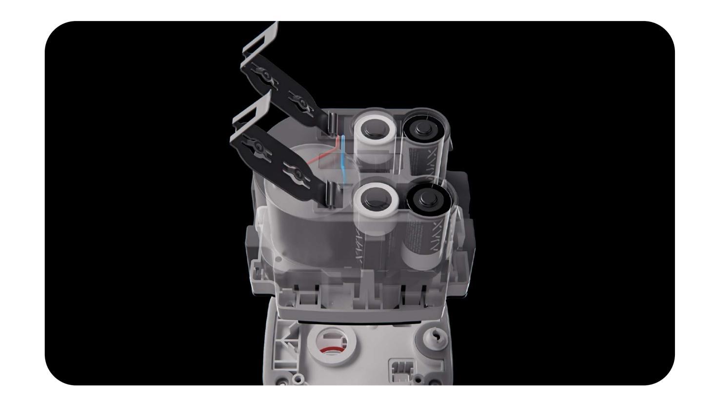
The electric actuator is mounted on the shutoff valve in four positions. The casing of the electric actuator does not need to be disassembled for installation. It is fixed on the valve with a mounting locker without tools. This way, there is no risk of damaging the electronics.
